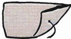
sandbag, 1/3 full, open end folded over - top view
